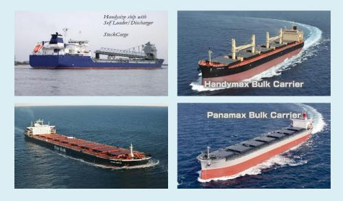
Both handysize and handymax carriers are ideal for shipments of different cargoes from smaller ports. Compared to very large bulk freighter; handysize and handymax can transport a greater variety of cargo types.
