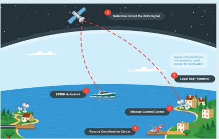
When the EPIRB is activated it transmits on 406.025 MHz. A digital signal is transmitted on 406.025 MHz. After the EPIRB is activated, the next passing satellite will detect the transmitted signal and relay it to an an-tenna at a ground station, called a LUT.
