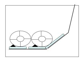
2 Wedges will be inserted for each coil.
