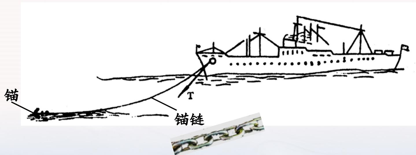
$$\sigma = \frac{N}{A} = \frac{P}{A} = \frac{196 \times 10^3}{2 \times \frac{\pi}{4} \times (49 \times 10^{-3})^2} \text{MPa} = 52 \text{MPa}$$
